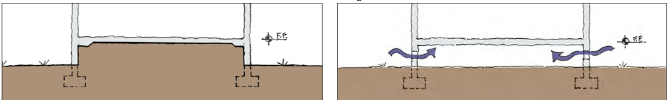
FIGURE 11 ALTERNATIVES TO FOUNDATIONS ON FILL
