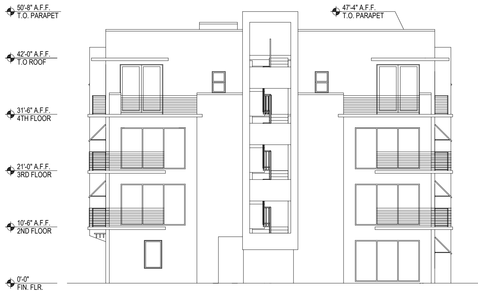
04 SOUTH ELEVATION BUILDINGS 1 & 3 SCALE: 3/32" = 1'-0"
