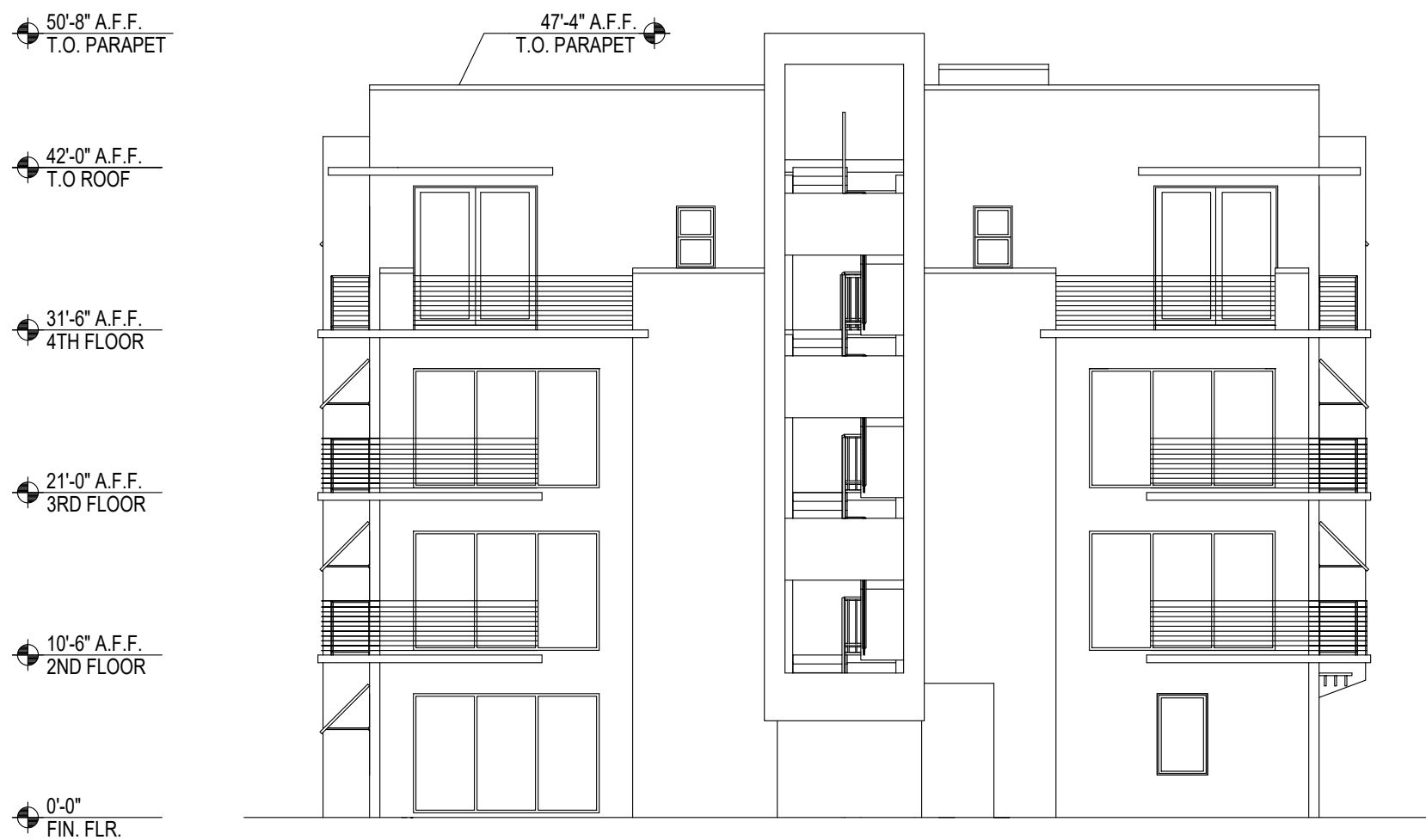
03 NORTH ELEVATION BUILDINGS 1 & 3 SCALE: 3/32" = 1'-0"
