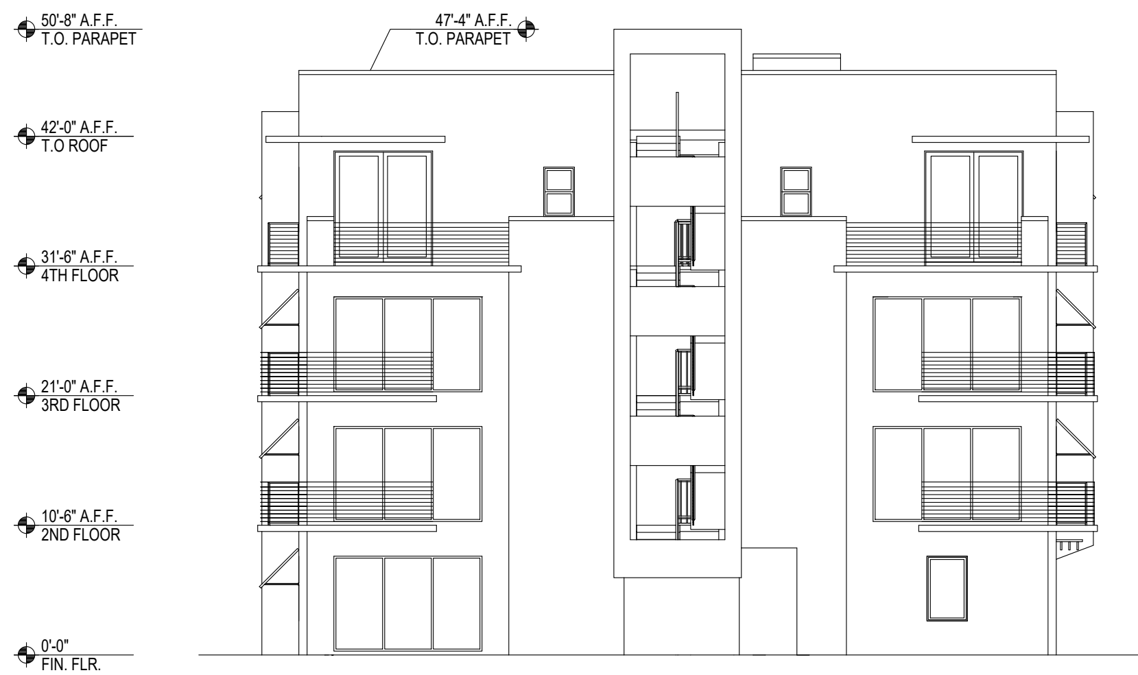
04 SOUTH ELEVATION BUILDINGS 2 & 4 SCALE: 3/32" = 1'-0"
