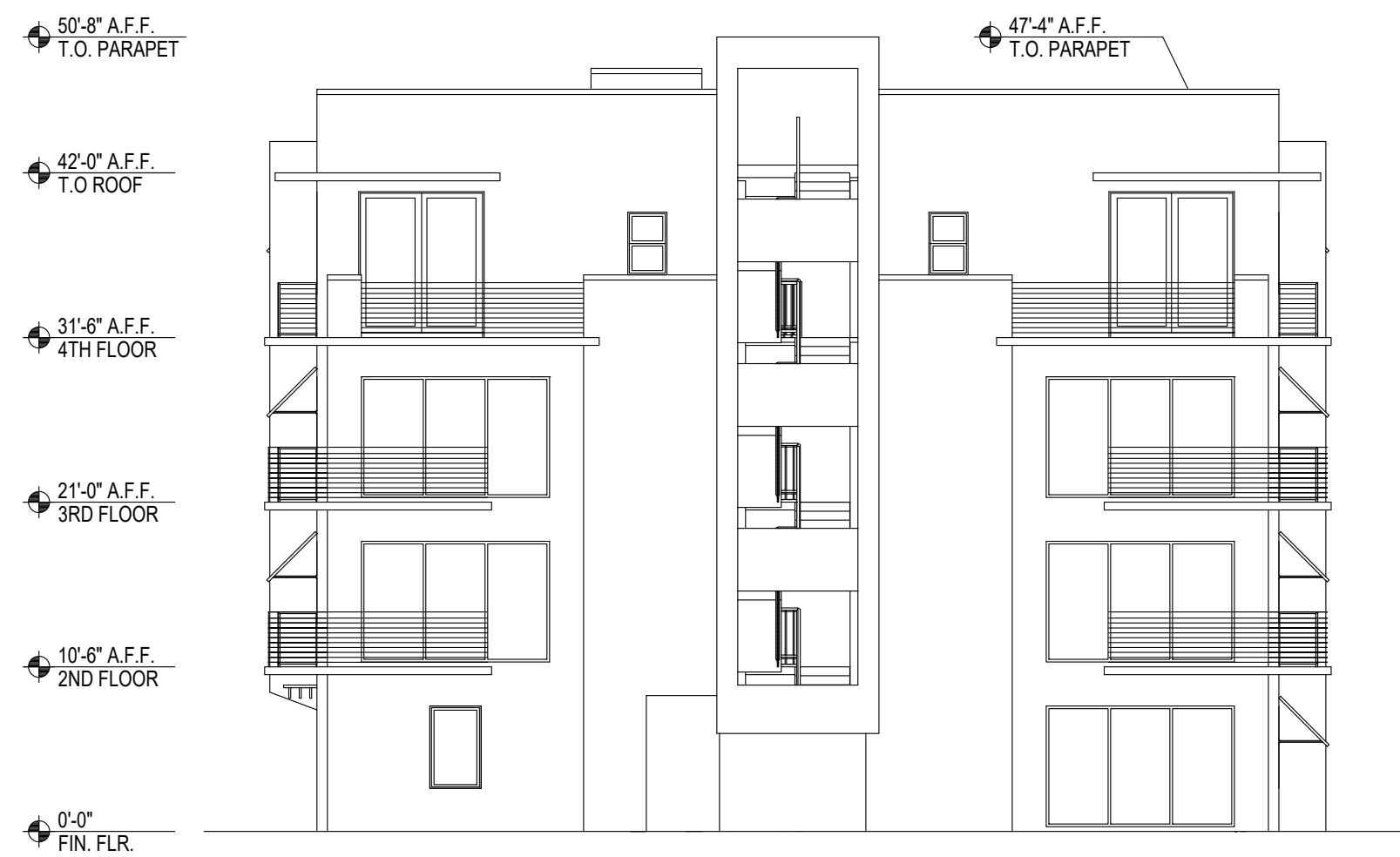
03 NORTH ELEVATION BUILDINGS 2 & 4 SCALE: 3/32" = 1'-0"
