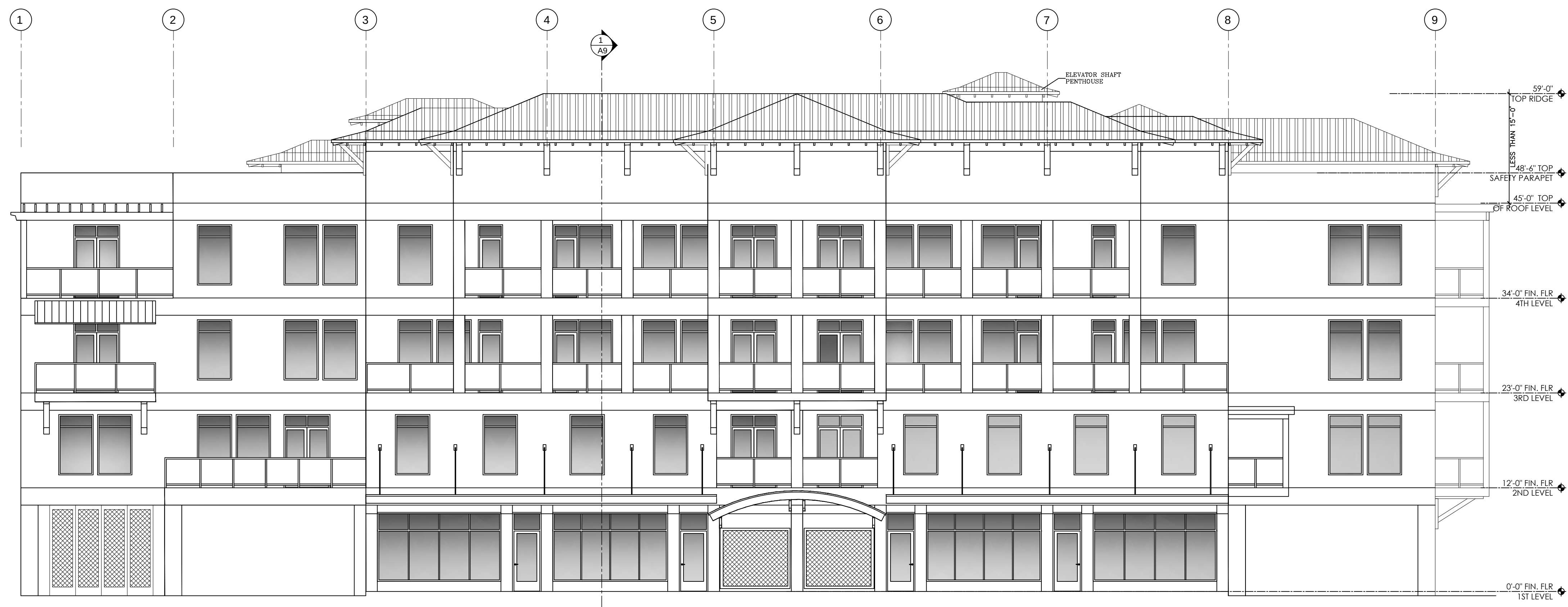
South Elevation SCALE: 1/8"=1'-0"
